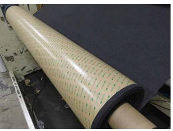
Applying adhesive backing to rolls
