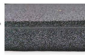
CGR laminated multiple plies of thin foam together to meet the OEM's custom thickness.multiple plies of thin foam together to meet the OEM's custom thickness.
