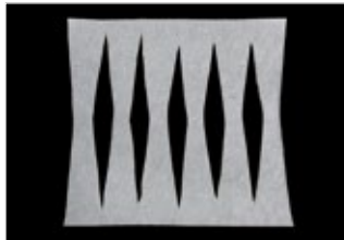
Figure 38: Form diamond-shaped cut out reverse gores in ArmaGel HT sheet.
